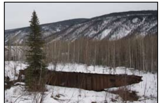
Derelict digging ladder from dismantled Dredge at Bear Creek.
