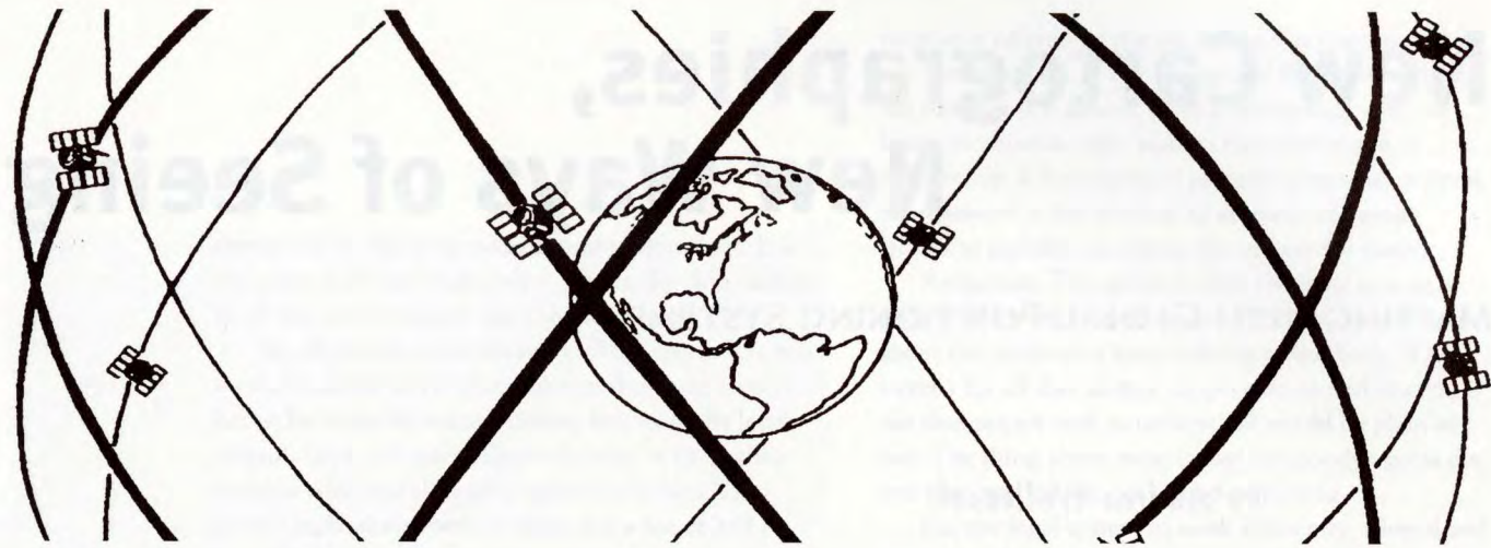
Twenty-four GPS Navstar Satellites orbit the earth in 23 hours and 56 minutes.
